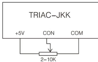
E, F, H types can be controlled by the manual control circuit, G type cannot be adjusted with the potentiometer
